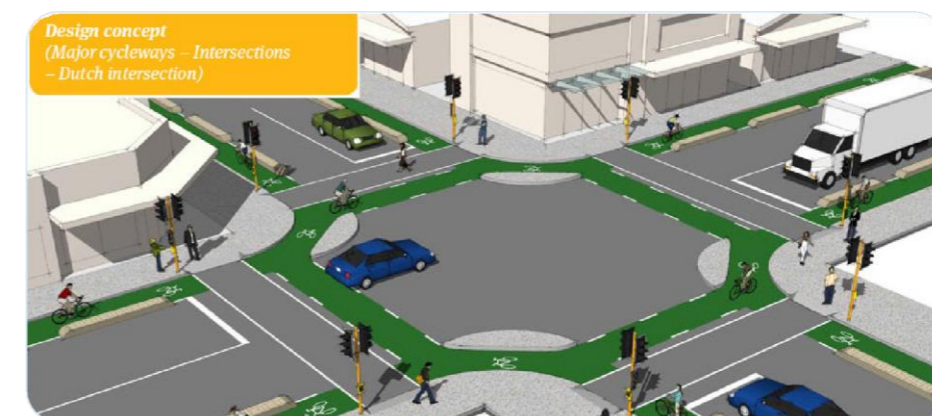
Figure 16: Key Infrastructure Elements of Protected Junction
